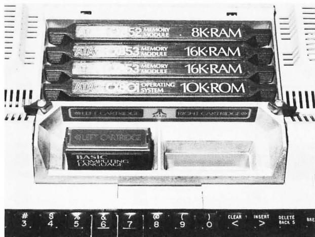
FIGURE 1.6 Cartridges containing read/write memory (RAM) and the ATARI's operating system (ROM).
