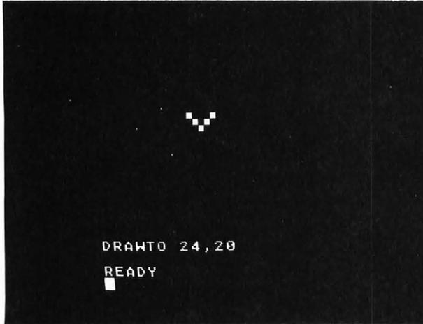
FIGURE 7.7 Plotting a line using `DRAWTO X,Y`.
