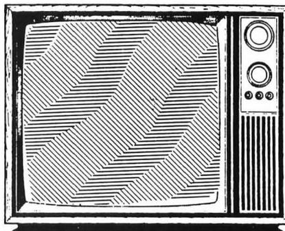
You probably do not have your computer's 2-3 switch and the TV turned to the same channel. Try switching channels and also check your computer switchbox on the back of the TV to make sure it's switched to "computer."
