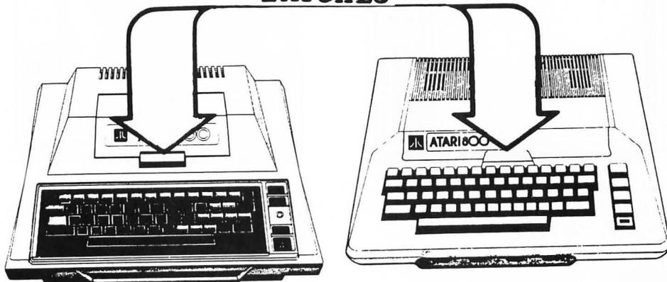
Next, with the label facing you, push the cartridge slowly but firmly down into the cartridge slot.
