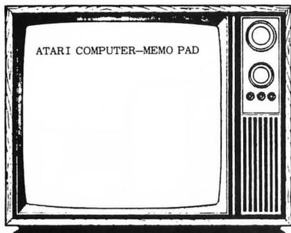
You might not have pressed the cartridge down firmly to the bottom of the slot.
