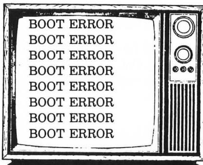
You probably have a disk drive connected and something elementary is wrong. For example, you could be using the wrong diskette or you might have left the disk drive door open. If you are just learning BASIC, you probably should turn the disk drive off. Turn the computer off, then on again. After introducing yourself to a little BASIC you can use your Disk Drive Manual to familiarize yourself with basic disk instructions. For starters work without a disk.
