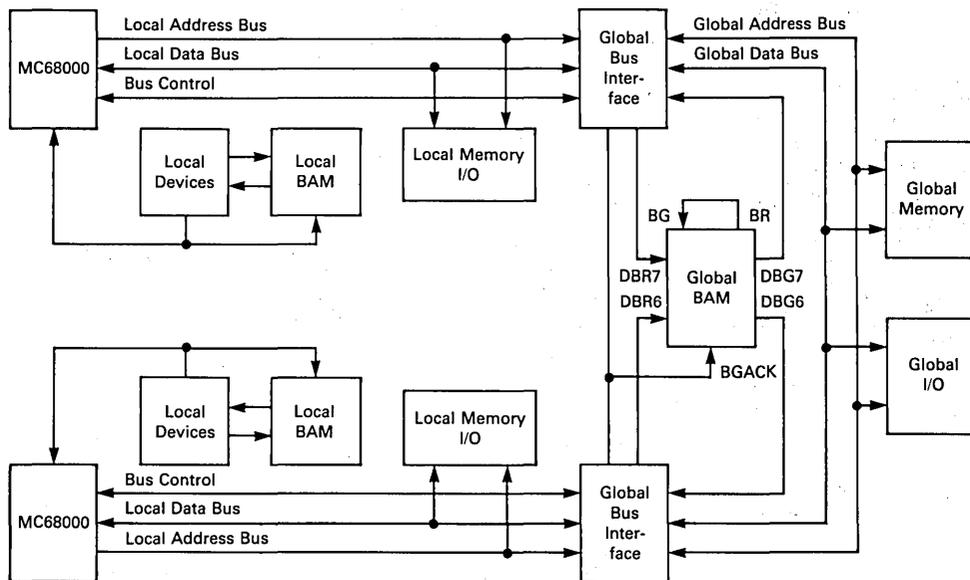
FIGURE 1 — MC68452 IN A MODERATELY COUPLED MULTI-PROCESSOR SYSTEM
