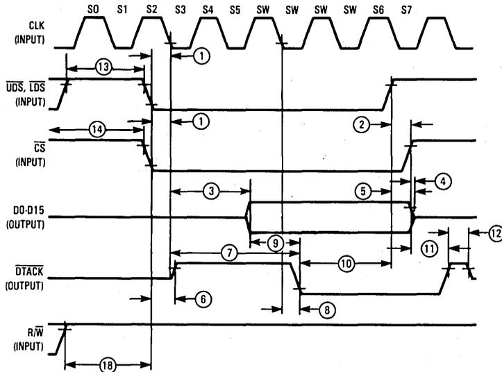
Figure 8. Host Processor Read Cycle Timing Diagram
