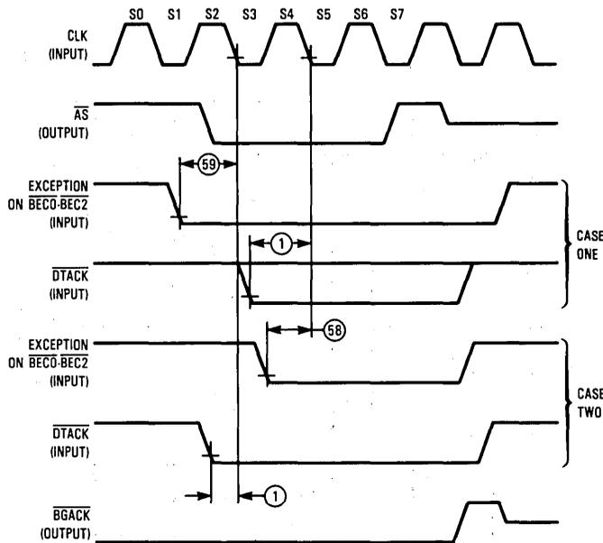
Two alternatives of  $\overline{DTACK}$  and exception. Case one has  $\overline{DTACK}$  occur after exception and case two has exception occur after  $\overline{DTACK}$ . Note that a HALT cycle can be terminated only by  $\overline{DTACK}$ .
