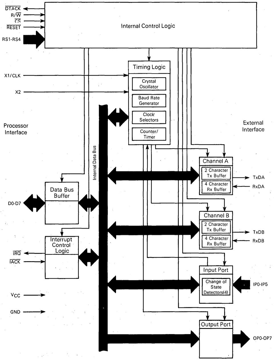
Figure 1. Block Diagram
