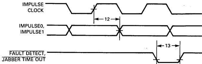
FIGURE 6-3 — IMPULSE OUTPUTS AND FAULT INPUTS
