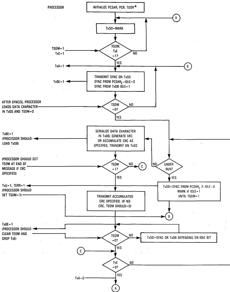
\* TxE must be asserted during initialization of PCSAR and PCR.
