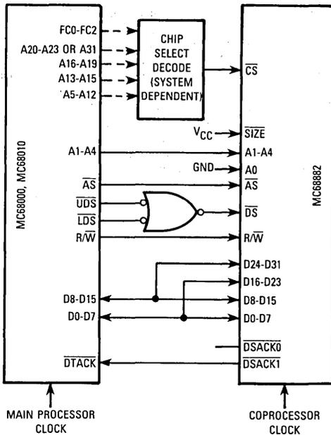
Figure 14. 16-Bit Data Bus Peripheral Processor Connection
