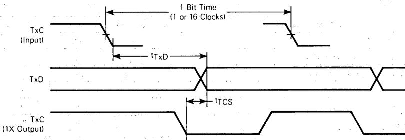
Figure 10. Transmit Timing
