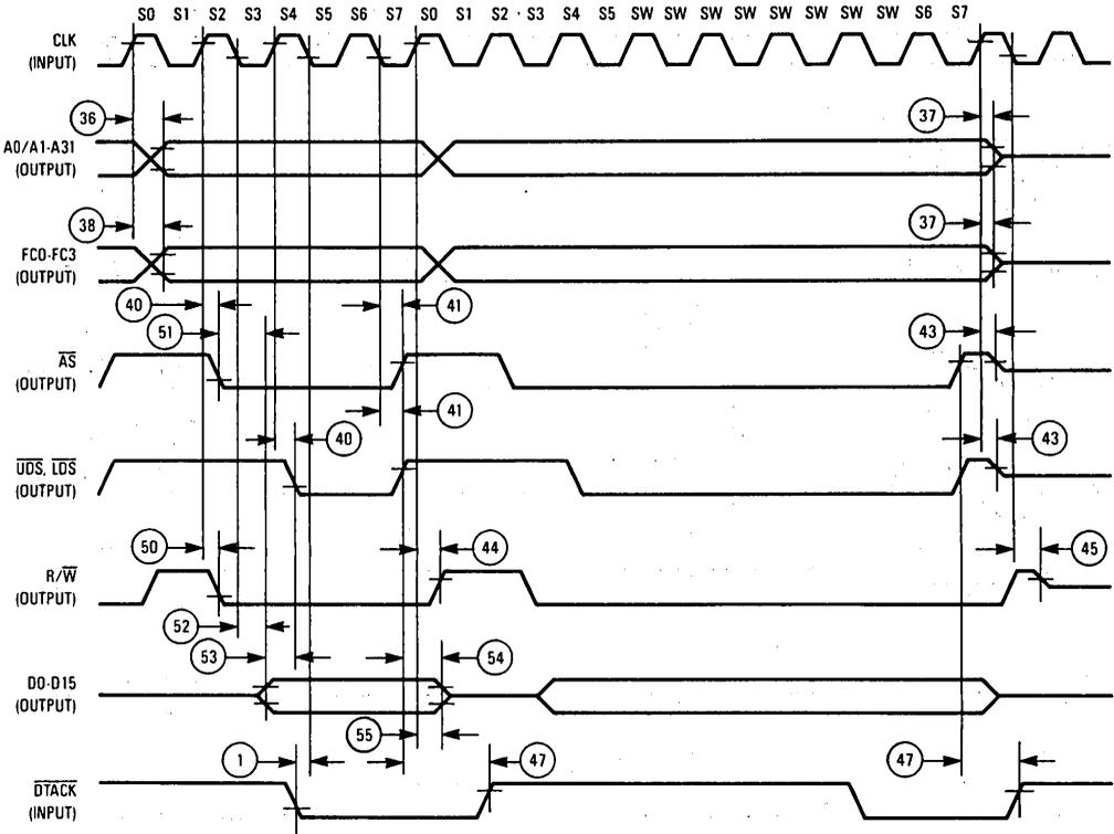
Figure 13. Write Cycle and Slow Write Cycle
