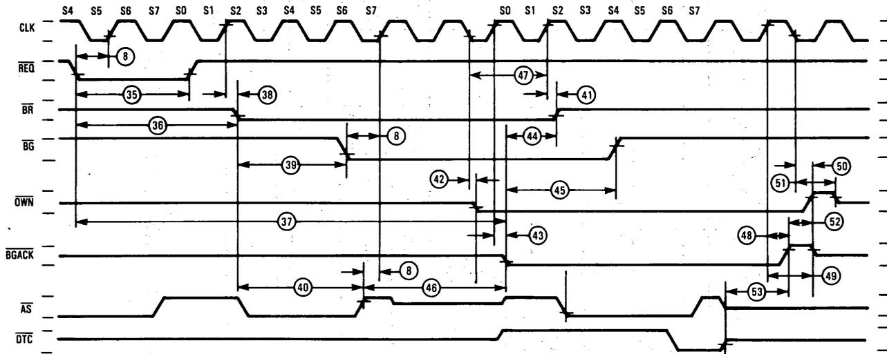
NOTE: Timing measurements are referenced to and from a low voltage of 0.8 volt and a high voltage of 2.0 volts, unless otherwise noted. The voltage swing through this range should start outside and pass through the range such that the rise or fall will be linear between 0.8 volt and 2.0 volts.
