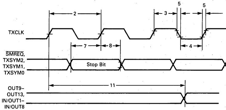
FIGURE 6-2 — SERIAL INTERFACE TRANSMITTER TIMING
