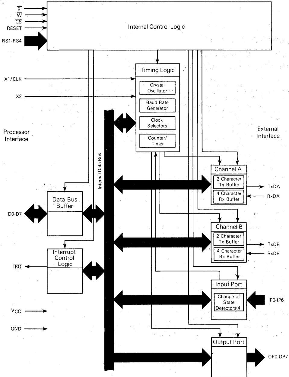
Figure 1. Block Diagram
