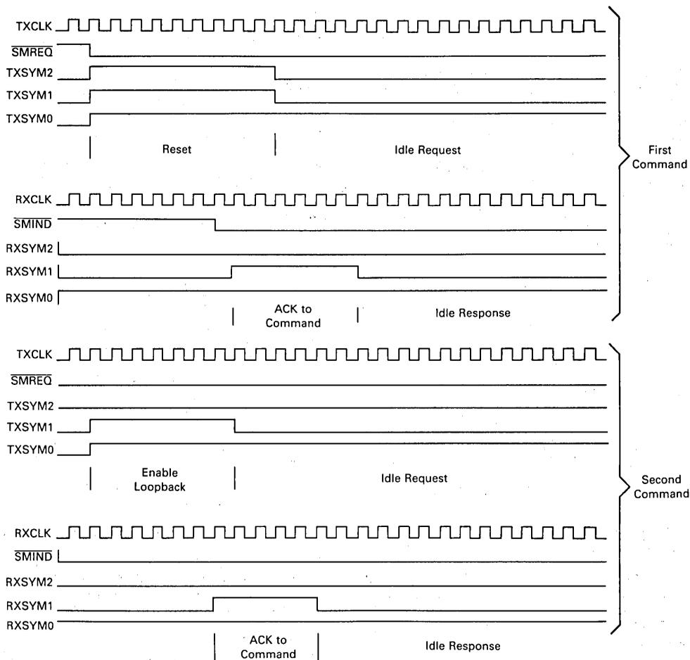
FIGURE 5-4 — STATION MANAGEMENT (SM) RESET AND LOOPBACK SEQUENCE
