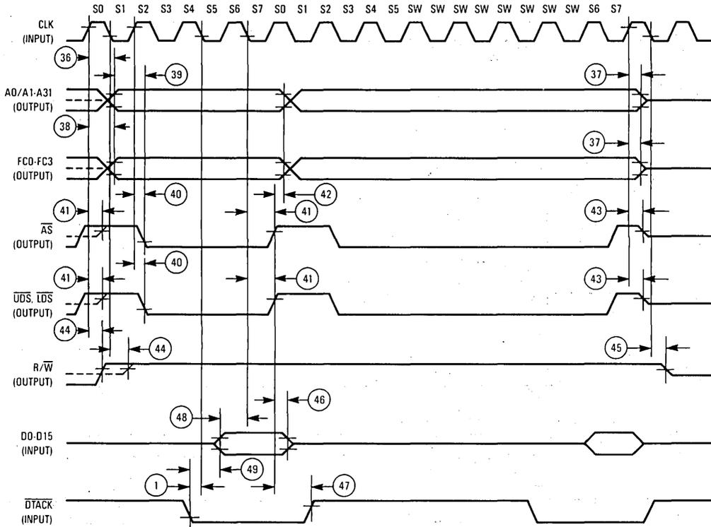
NOTE: The solid lines assume that the communication controller was bus master on the last cycle. The dotted lines assume that there was a different bus master.
