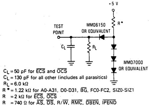
Figure 9. Test Load
