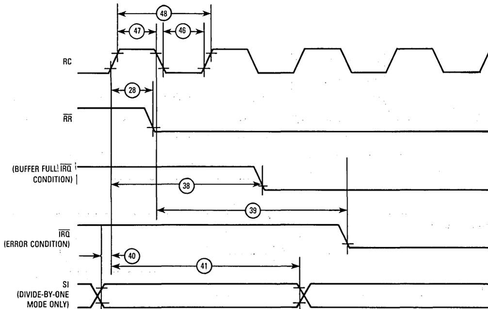
Figure 17. Receiver Timing
