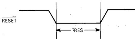
Figure 3. RESET Timing
