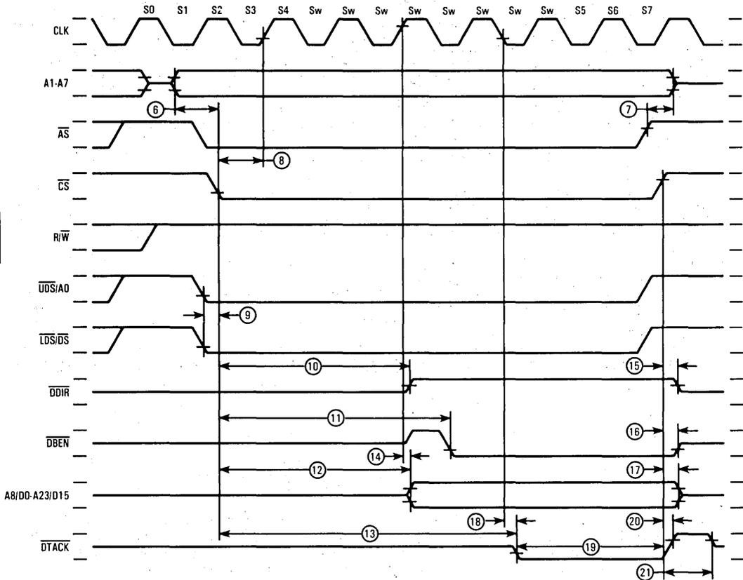
NOTE: Timing measurements are referenced to and from a low voltage of 0.8 volt and a high voltage of 2.0 volts, unless otherwise noted. The voltage swing through this range should start outside and pass through the range such that the rise or fall will be linear between 0.8 volt and 2.0 volts.
