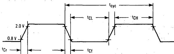
NOTE: Timing measurements are referenced to and from a low voltage of 0.8 volt and high voltage of 2.0 volts, unless otherwise noted. The voltage swing through this range should start outside and pass through the range such that the rise or fall will be linear between 0.8 volt and 2.0 volts.
