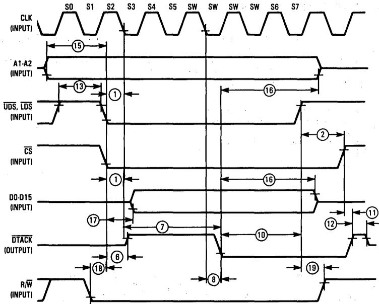
Figure 9. Host Processor Write Cycle Timing Diagram
