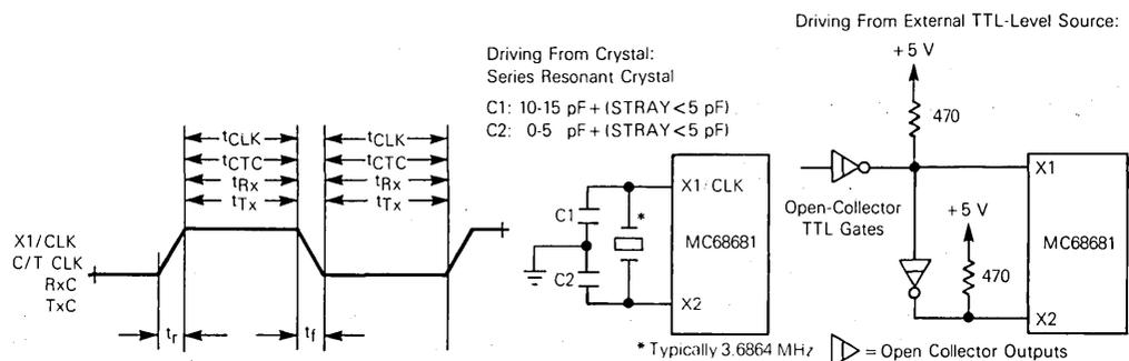
NOTE: Board layout should be such that the crystal and capacitor(s) are as close as possible to the pins of the DUART to minimize stray capacitance. Also, crystal series resistance should be less than 180 ohms.
