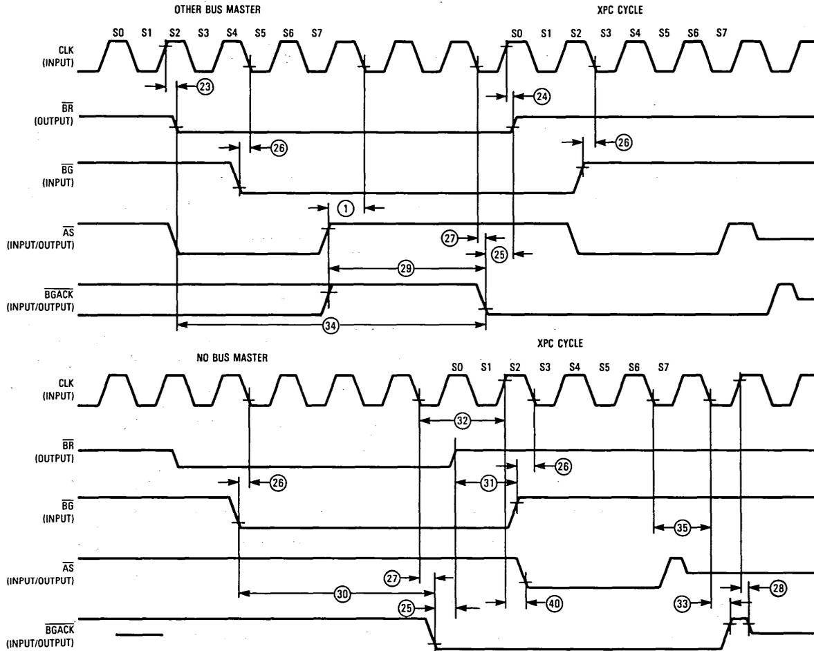
Figure 11. Bus Arbitration Timing Diagram
