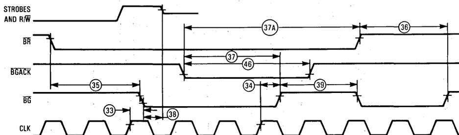
NOTE: Setup time to the clock (#47) for the asynchronous inputs  $\overline{BERR}$ ,  $\overline{BGACK}$ ,  $\overline{BR}$ ,  $\overline{DTACK}$ ,  $\overline{IPL0}$ - $\overline{IPL2}$ , and  $\overline{VPA}$  guarantees their recognition at the next falling edge of the clock.
