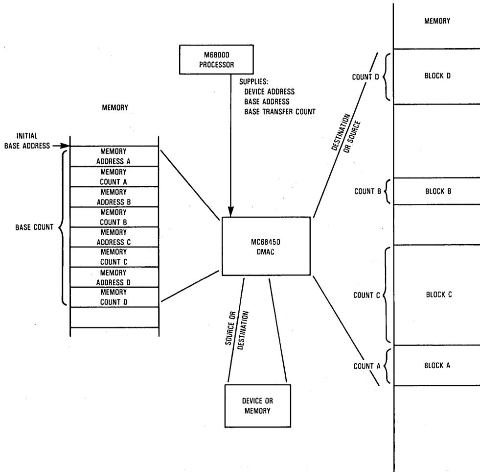
Figure 6. Array Chain Transfer
