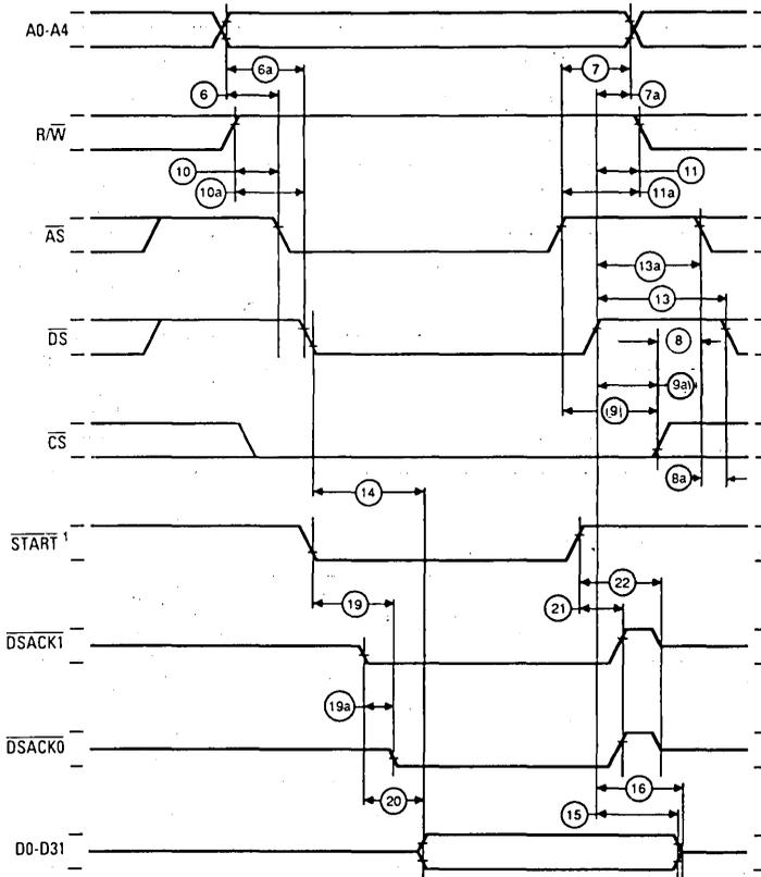
Figure 18. Asynchronous Read Cycle Timing Diagram
