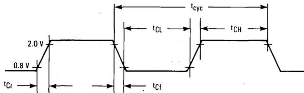
NOTE: Timing measurements are referenced to and from a low voltage of 0.8 volt and high a voltage of 2.0 volts, unless otherwise noted. The voltage swing through this range should start outside and pass through the range such that the rise or fall will be linear between 0.8 volt and 2.0 volts.
