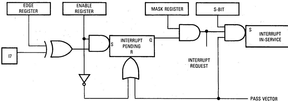
Figure 6. Conceptual Circuits of an Interrupt Channel
