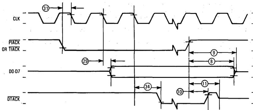
NOTE: Timing measurements are referenced to and from a low voltage of 0.8 volt and a high voltage of 2.0 volts, unless otherwise noted.
