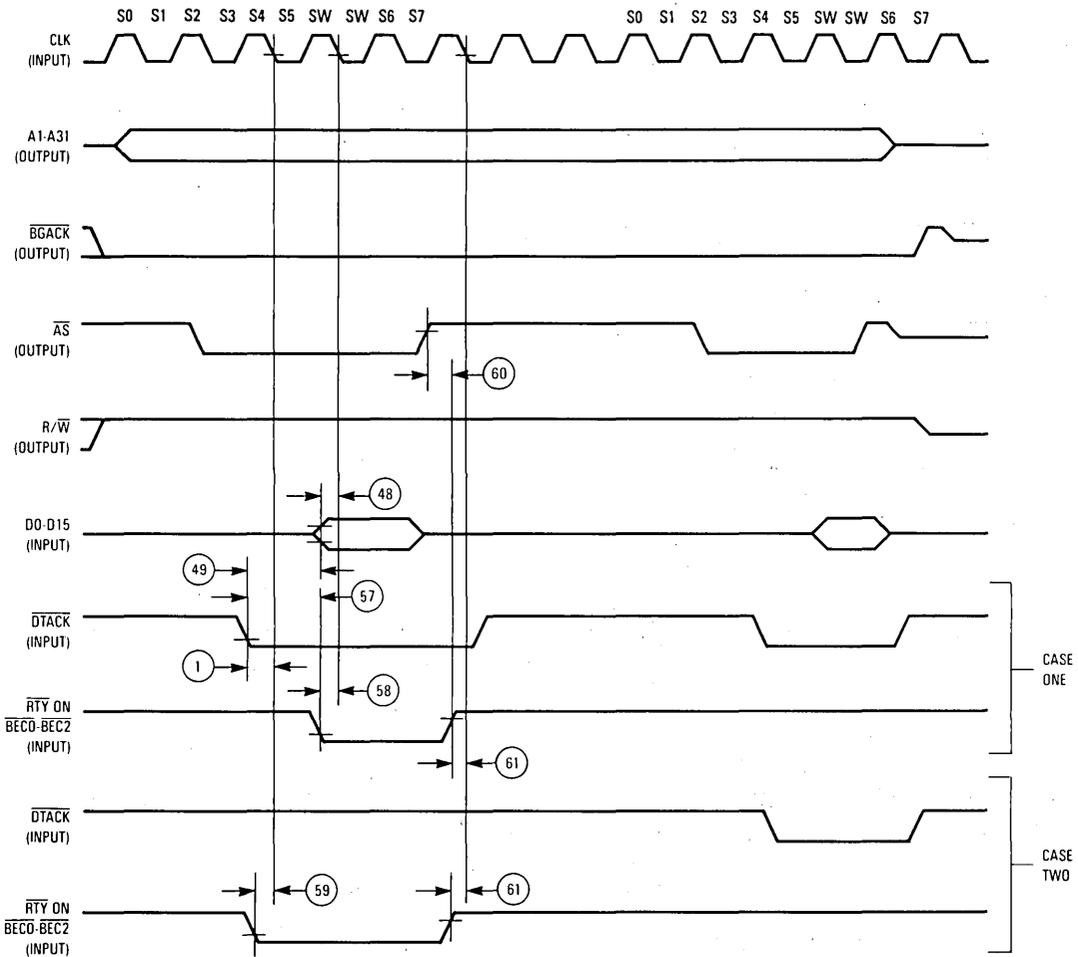
CASE ONE: If  $\overline{DTACK}$  satisfies 1 then 48 and 58 are required. If  $\overline{DTACK}$  is active but does not satisfy 1 then 49 and 57 are required.
