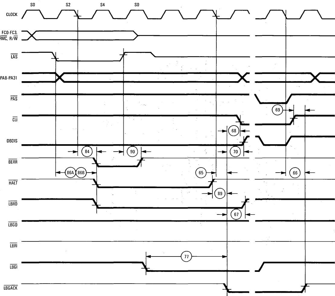
Figure 12. Logical Master Relinquish and Retry Timing Diagram
