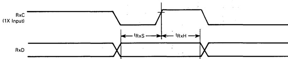
Figure 9. Receive Timing
