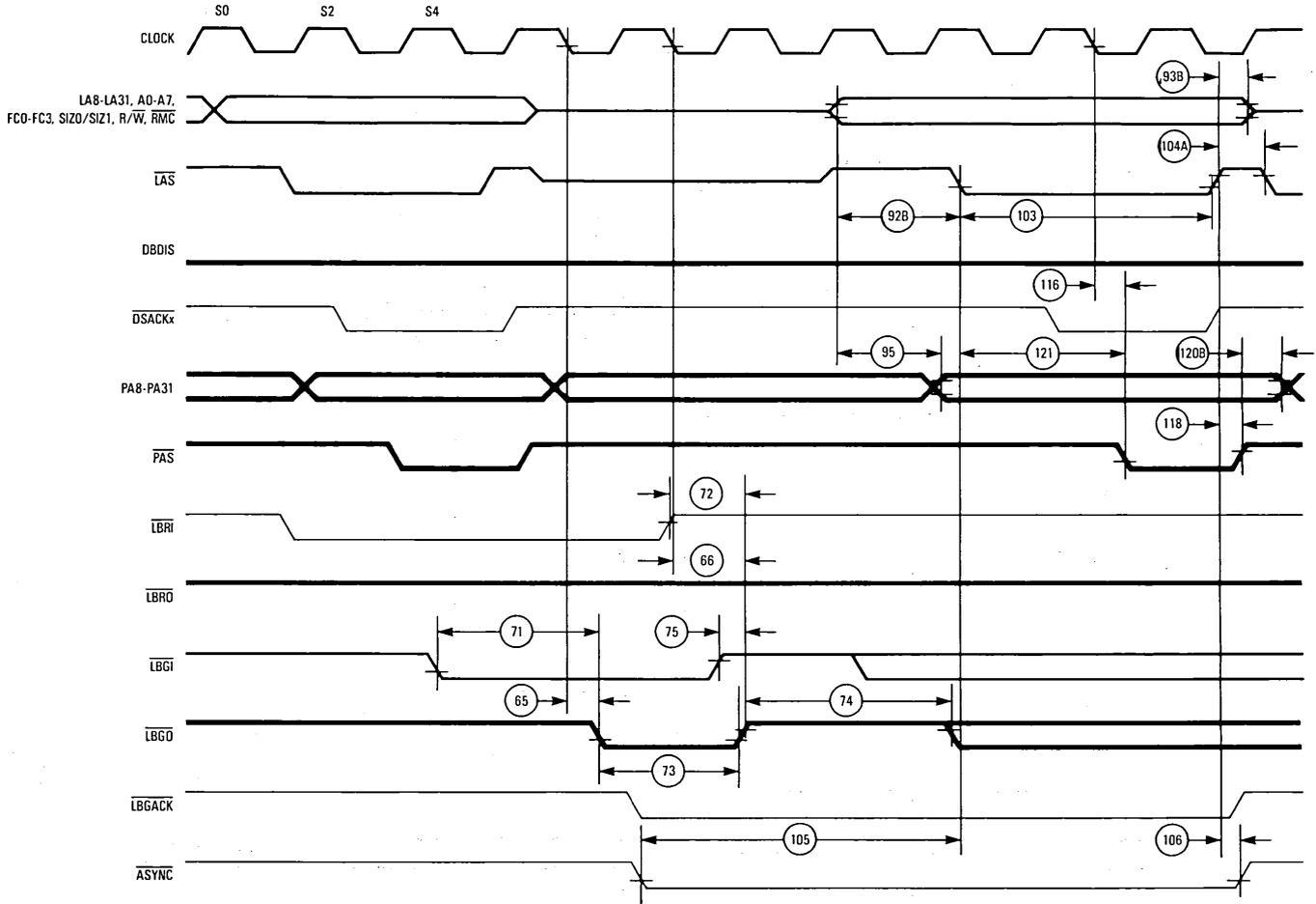
Figure 13. Logical Bus Arbitration by Asynchronous Master Timing Diagram
