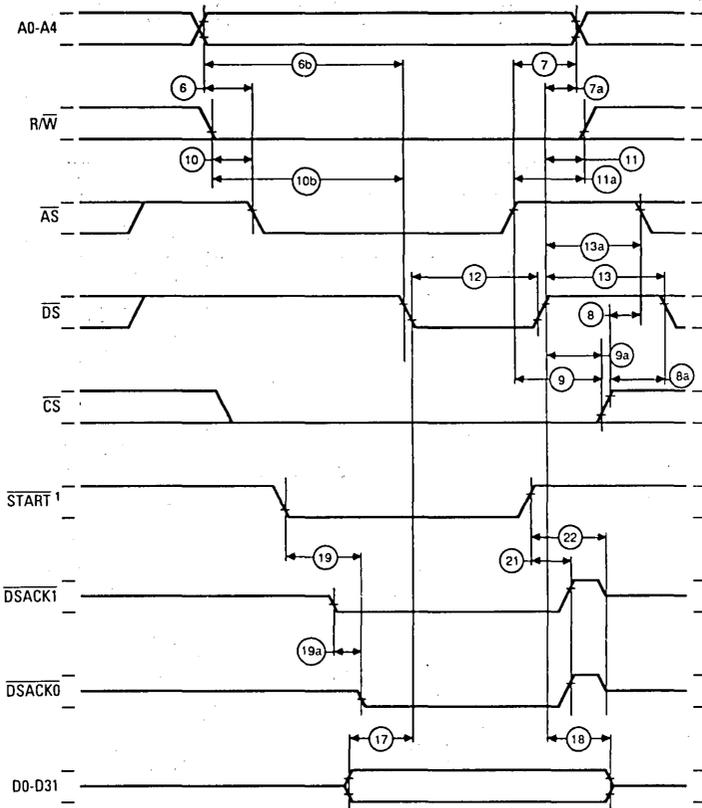
Figure 18. Asynchronous Write-Cycle Timing Diagram
