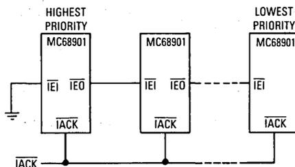
Figure 5. Daisy-Chaind Interrupt Structure
