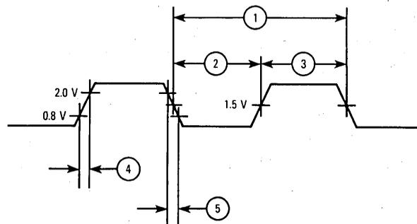
Figure 9. Clock Input Timing Diagram
