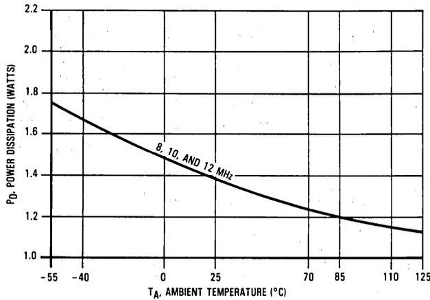
Figure 11. MC68440/MC68442 Power Dissipation vs Ambient Temperature
