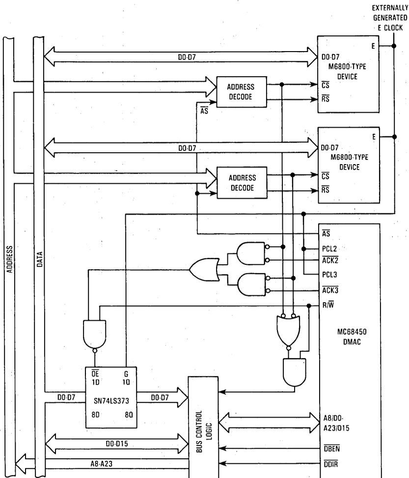
Figure 2. Typical System Configuration with M6800-Type Peripheral Devices
