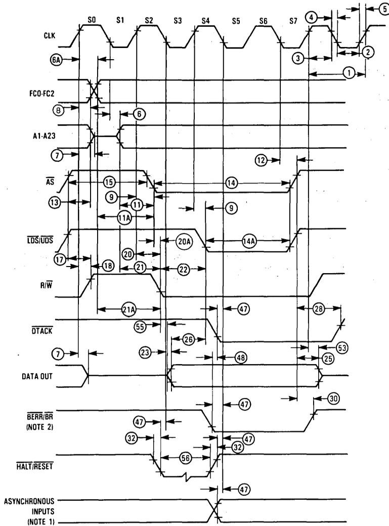
Figure 9. MC68008 Write-Cycle Timing Diagram
