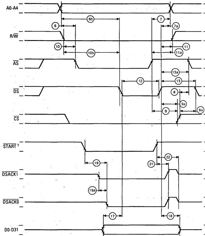
Figure 19. Asynchronous Write-Cycle Timing Diagram
