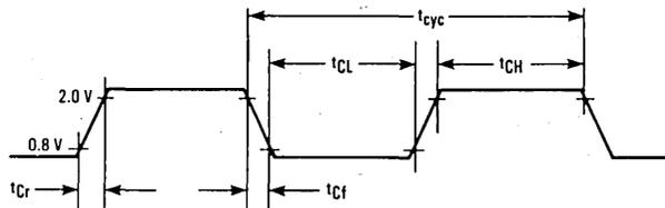
NOTE: Timing measurements are referenced to and from a low voltage of 0.8 volts and a high voltage of 2.0 volts, unless otherwise noted. The voltage swing through this range should start outside and pass through the range such that the rise or fall will be linear between 0.8 volts and 2.0 volts.
