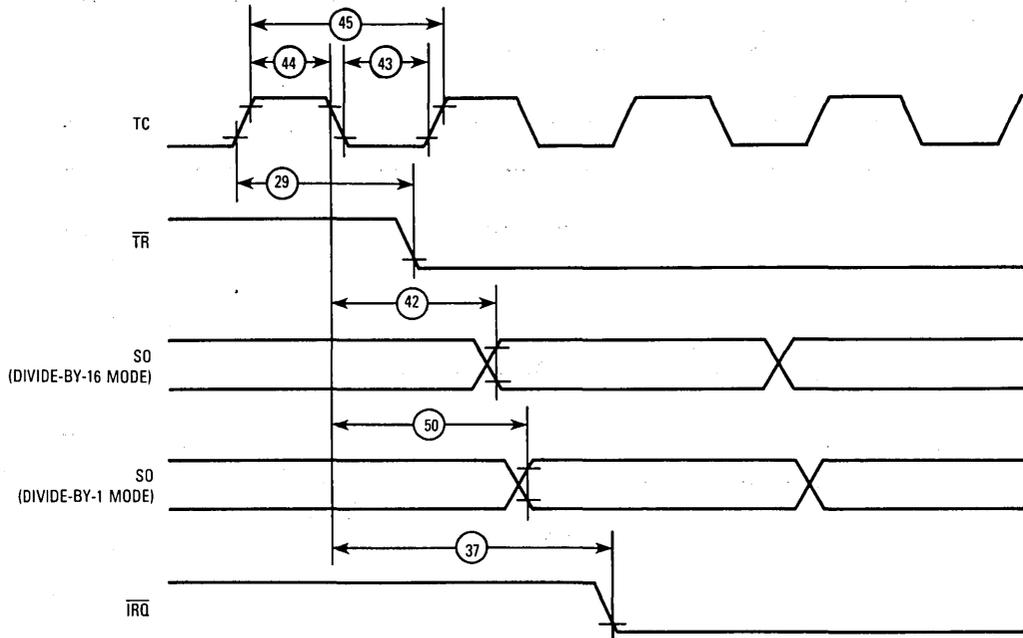
Figure 18. Transmitter Timing
