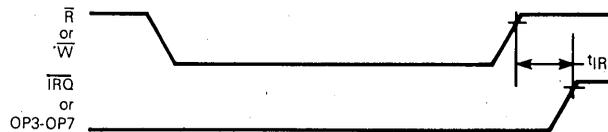
Figure 6. Interrupt Timing
