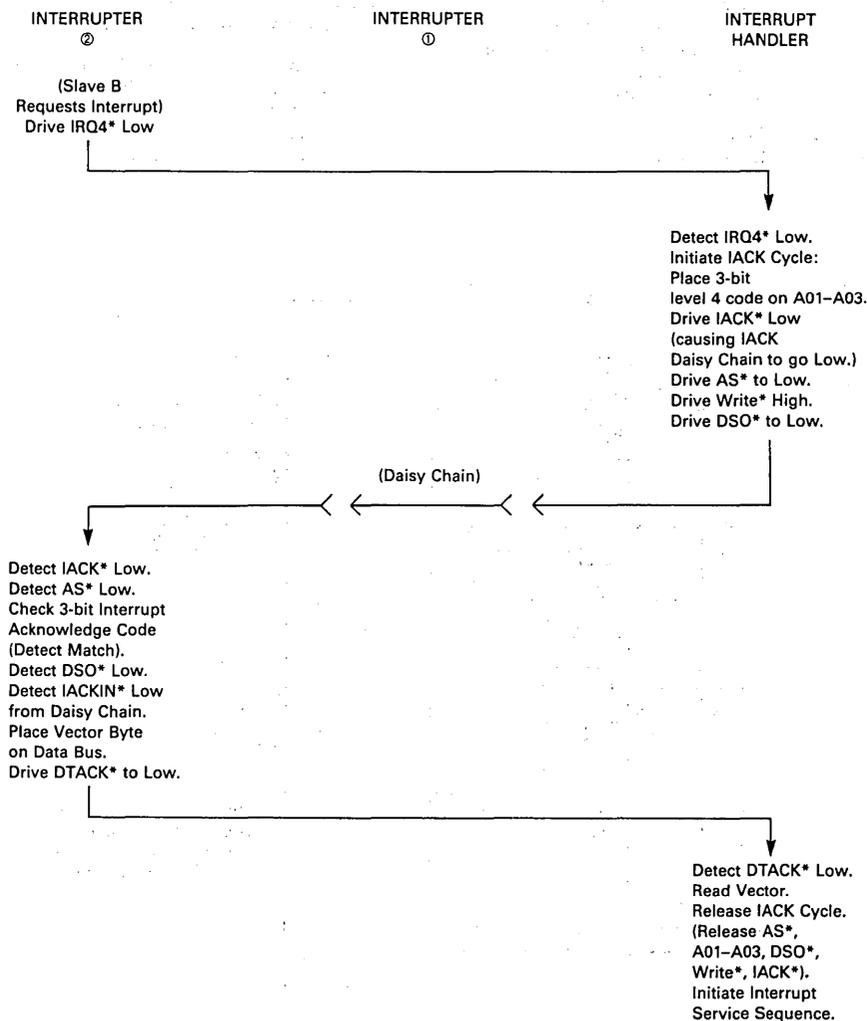
FIGURE 6 — INTERRUPT REQUEST AND ACKNOWLEDGE OPERATION FLOW DIAGRAM
