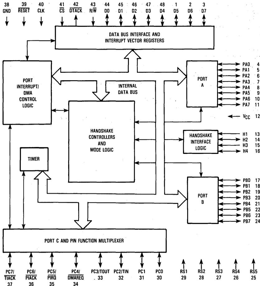
Figure 1. Block Diagram
