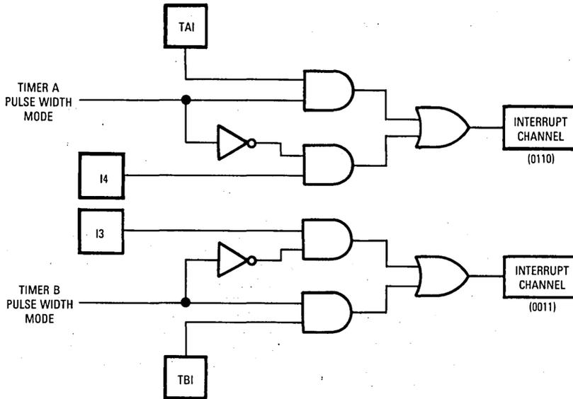
Figure 7. Conceptual Circuit of Interrupt Source Selection
