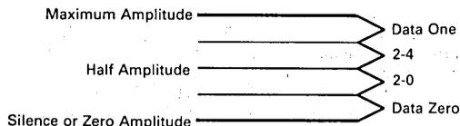
This technique assumes that the error was caused by a small amount of noise which pushed the data out of its normal range into the nearest non-data range. In order to determine if a non-data is part of an end delimiter or not, four rules are used: (See 2.2.2 AGC HOLD for bit positions.)
