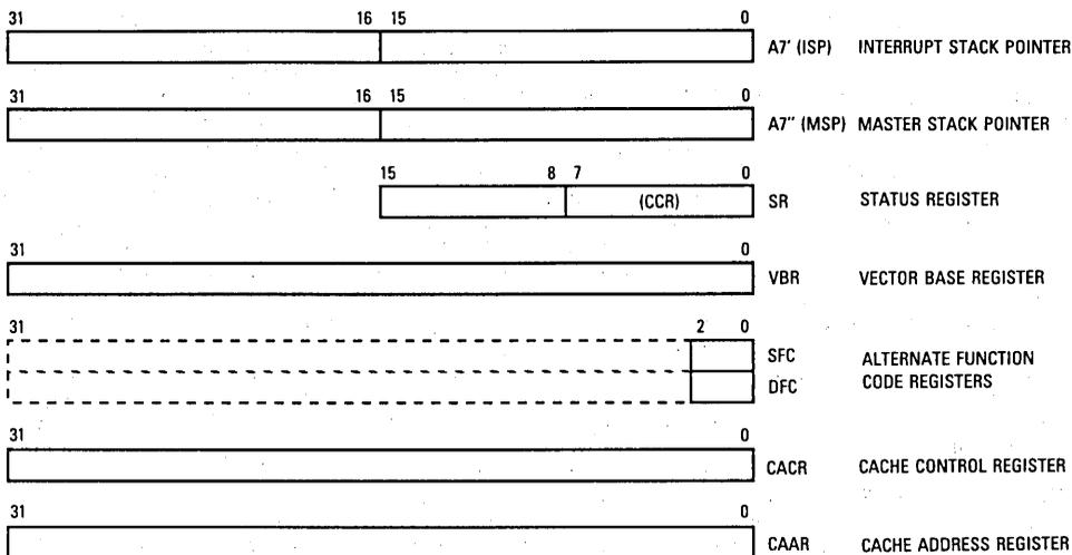
Figure 3. Supervisor Programming Model Supplement
