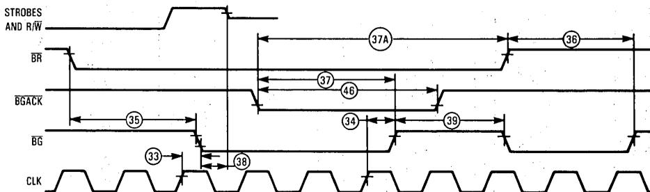
NOTE: Setup time to the clock (#47) for the asynchronous inputs  $\overline{BERR}$ ,  $\overline{BGACK}$ ,  $\overline{BR}$ ,  $\overline{DTACK}$ ,  $IPL0-IPL2$  and  $\overline{VPA}$  guarantees their recognition at the next falling edge of the clock.
