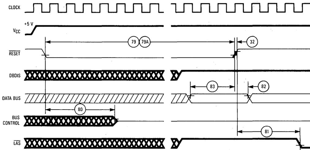
Figure 17. Reset and Mode Select Timing Diagram
