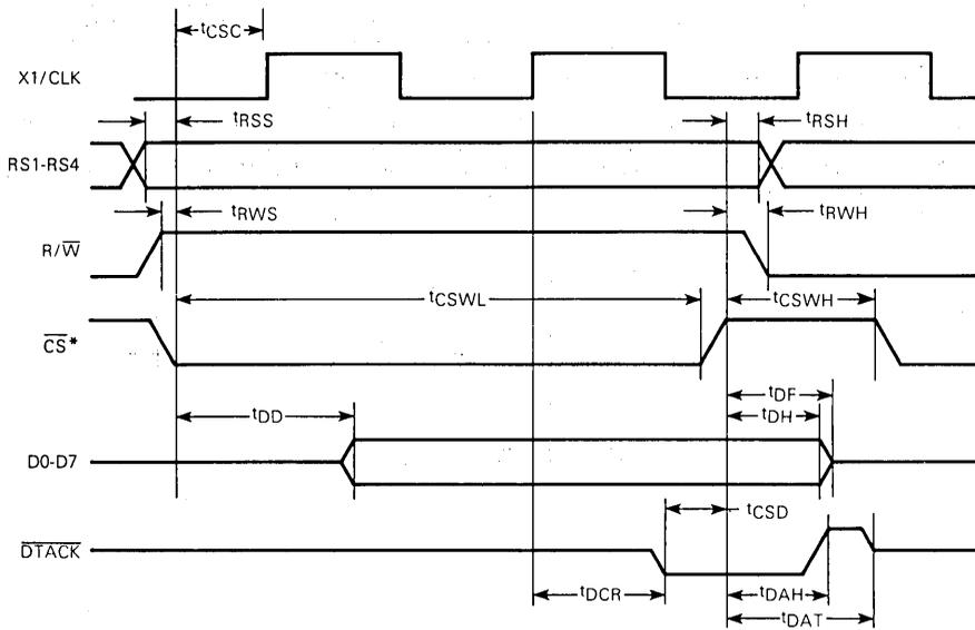
\* $\overline{CS}$  and  $\overline{IACK}$  should not be asserted simultaneously.
