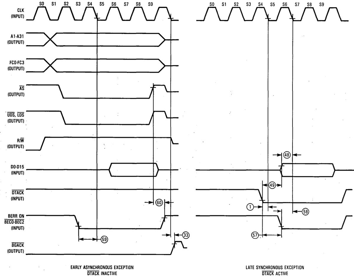
Figure 15. Read Cycle with Bus Error Timing Diagram
