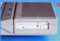
The case can now be screwed back together. Run the AUTO program and the CPX or accessory to format your first high density disk.
