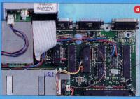
Make sure there is enough clearance for the plugs when the drive is in place. The brown wire is connected to pin two on the drive itself.
