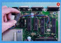
The controller in this machine is the VL1772. so it is being changed for a WD1772 02-02 chip. The original chip has been removed and a socket has been soldered in place.
