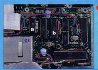
Switch the power off and open vour ST. Remove the board from the case, locate the floppy disk drive controller (a) and the sound chip (b).
