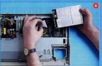
When everything is working, disconnect the power and reassemble the computer. The brown lead can be connected to the disk drive itself or to the lead that plugs into the back of it.
