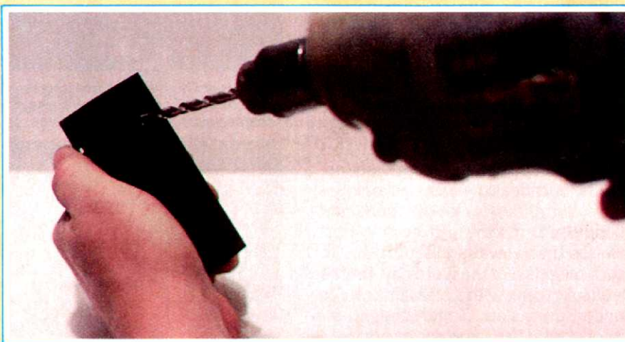
FIGURE 5: With the \frac{1}{4} " drill bit, drill a hole through the modulator cover, approximately \frac{1}{2} " from the screw hole.
