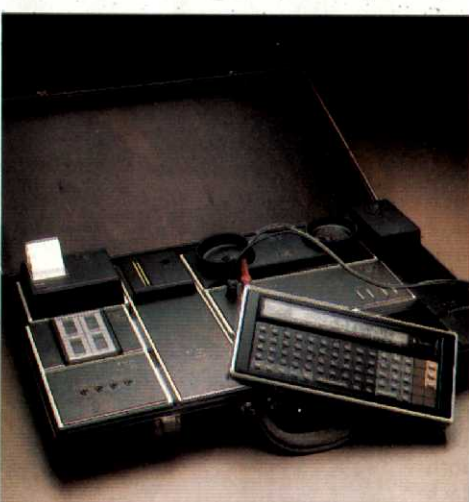
Quasar creates a briefcase computer with its Micro-Information System (about $2000). A hand-held computer terminal and optional programmable memory, printer, telephone modem connect to make a powerful computer.
