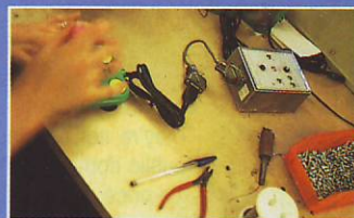
■ Every joystick is tested by being plugged into a box of LEDs. Only if the right connections are made will the stick be packaged.
