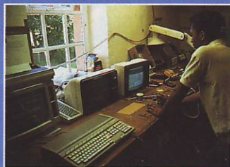
■ One in 10 joysticks are tested on games in the games room just to make certain that there are no faulty batches. With a new design every stick is tested.
