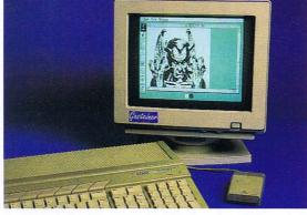
the top of the screen, however, and the Desktop display has an annoying upwardly curved edge. The only picture controls on the front of the monitor are brightness and contrast. The rear of the machine boasts a couple of controls for adjusting the vertical image size and horizontal phase as well as two holes for other controls that have to be adjusted with a screwdriver. These two controls are for the focus and the sub-brightness they are pre-set at the factory and should not need altering.
