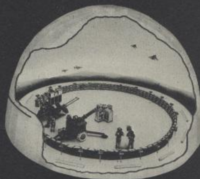
Above: Anti-aircraft training using computer-linked light projection. Below: A cutaway view of the anti-aircraft trainer.
