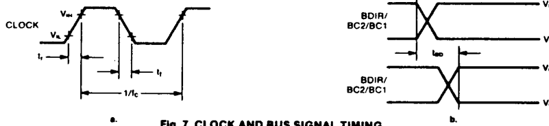
Fig. 7 CLOCK AND BUS SIGNAL TIMING
