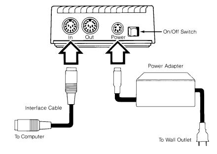
**Warning:** When setting up your computer system, place your disk drive at least 12 inches away from your monitor. Monitors emit a magnetic field that can damage information recorded on disks.
