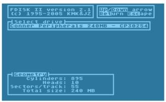
(which means that the FDISK2 is unable to find the interface), please turn the power off, check the connection between the interface and the computer, then try again. Check the Master/Slave jumper position on the drive.
