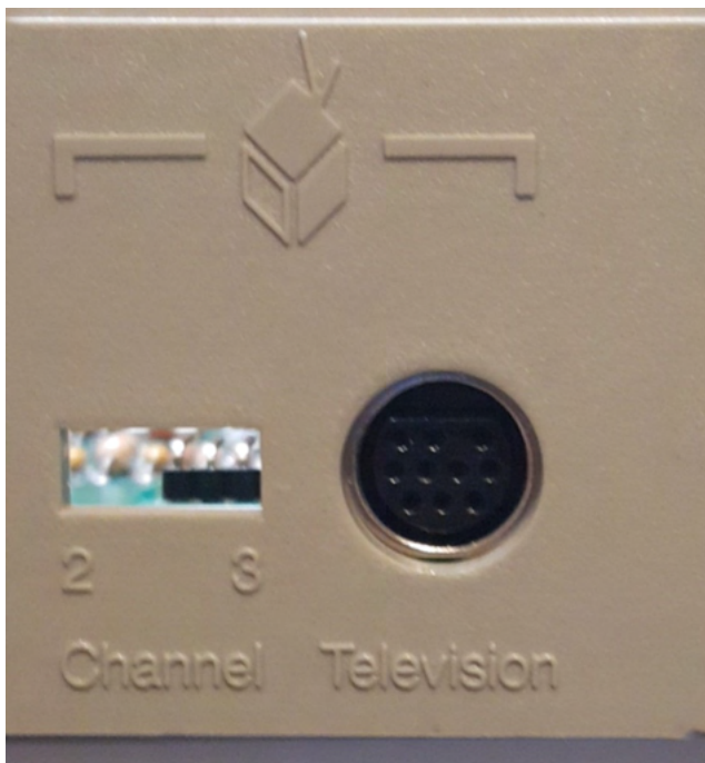
Rear view of the Atari XE with SAVO XE installed and Sega Saturn AV socket instead of the RF modulator antenna.
