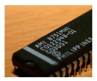
2. If POKEY CHIP is socketed, remove it from socket. If it is not socketed, You have to desolder it and solder back into it's place precision 40 pin socket You just found in SSTEREO set.
